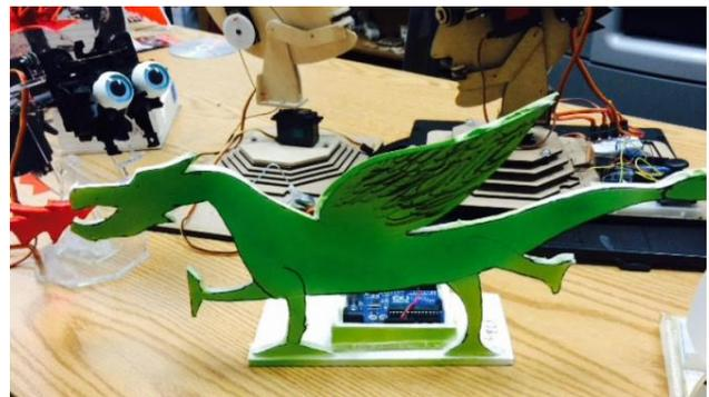
**Figure 1. Simple Green Dragon Robot programmed to appear to breathe flames that move back and forth. Made from scratch using an Arduino, LED light, servo, and foam core.**
