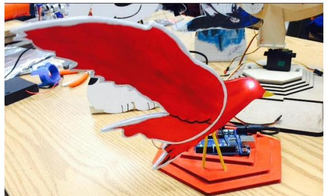
**Figure 3. Red Cardinal Bird Robot fabricated on a CNC laser cutter and programmed with Arduino to control a servo.**
