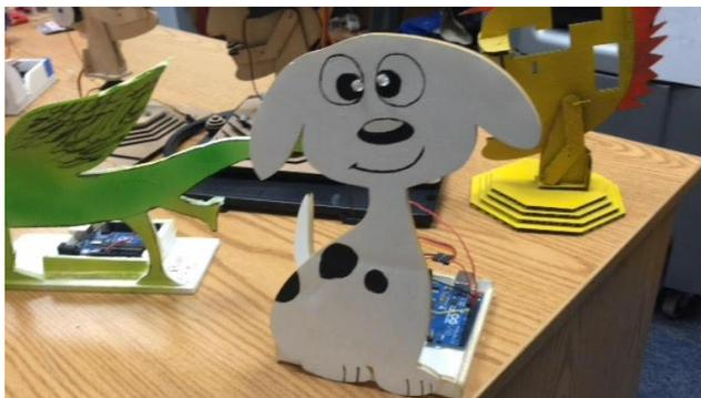
**Figure 4. Complex robot puppy fabricated on a CNC laser cutter programmed to blink eyes and tail to wag.**
