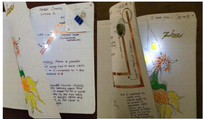
**Figure 2. Electric Notebook made with simple and parallel copper tape circuits, circuit stickers, and 3-volt coin battery.**
